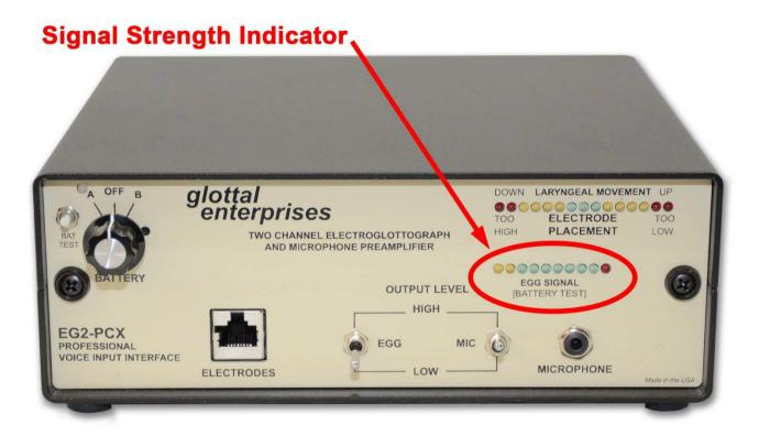
• Signal Strength Indicator allows you to separate between a good signal and those that are too low for accurate waveform representation.
